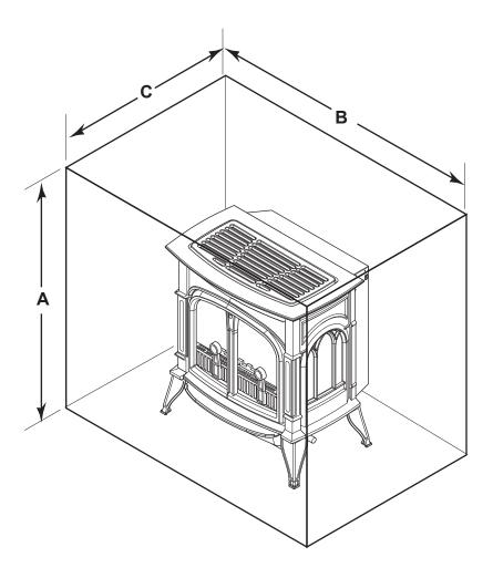
Figure 5 - Placing Stove in Alcove
